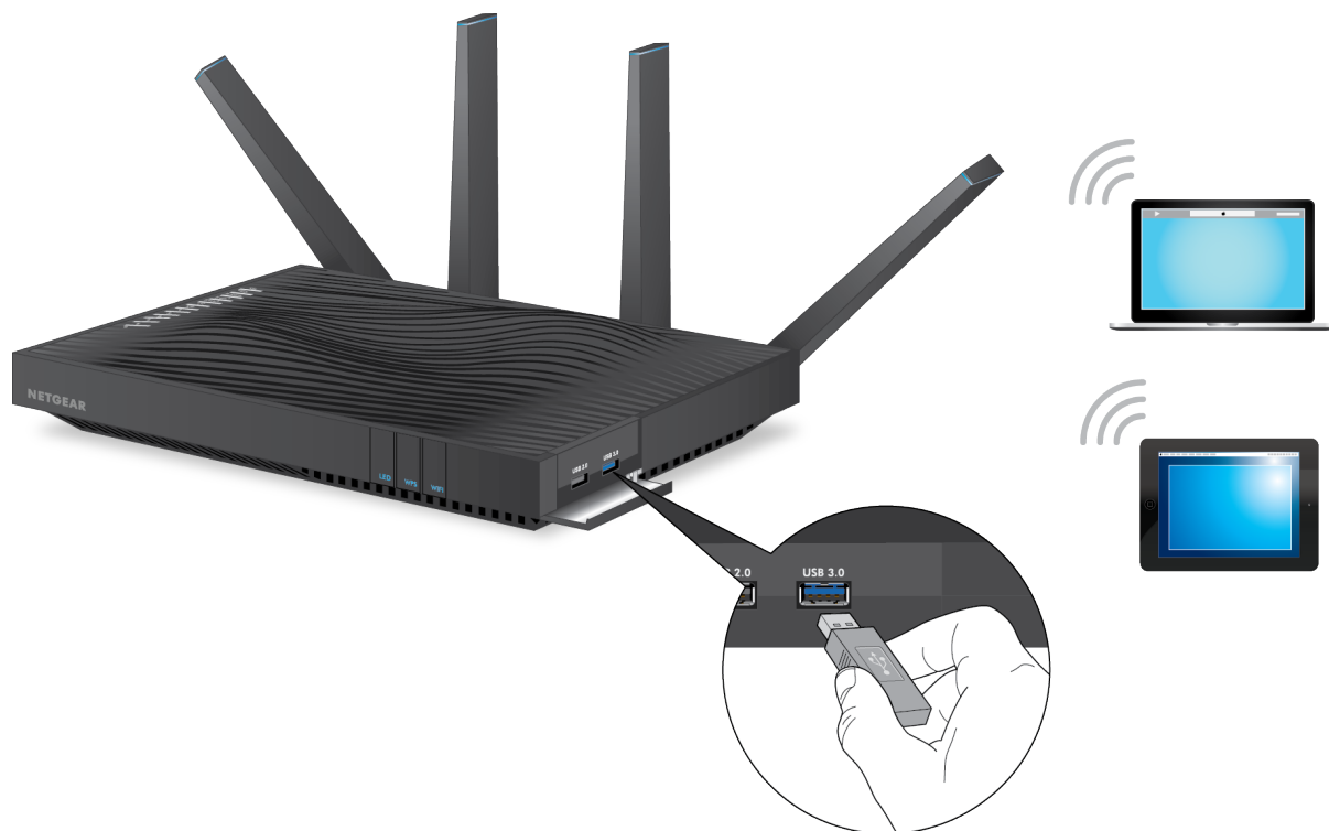
Figure 3. A USB 3.0 port and a USB 2.0 port are located on the right
